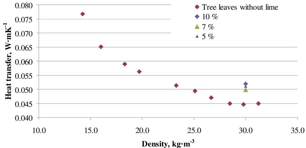
Fig. 3. Tree leaves heat transfer change curve depends on density and lime admixture
