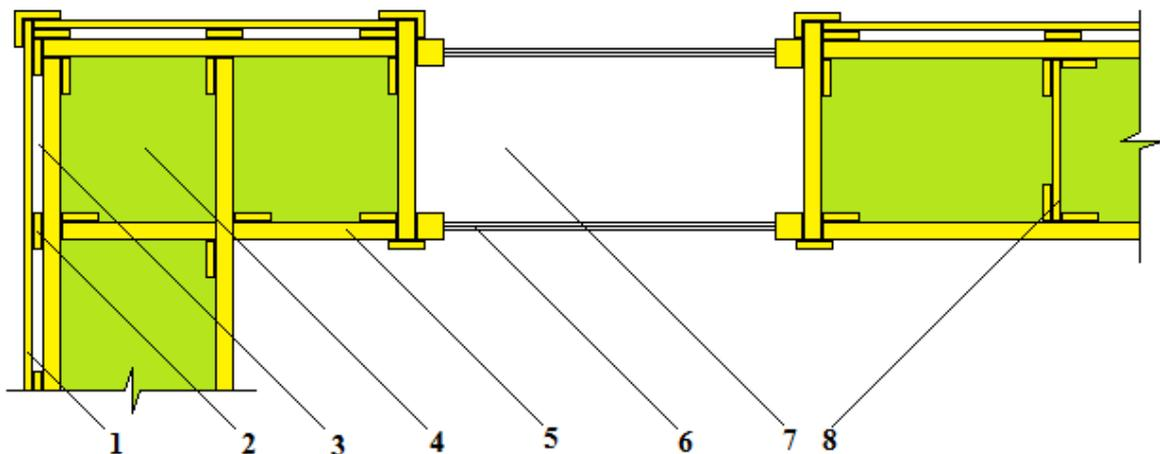
Fig. 4. Wood wall construction with filling heat insulation material: 1 – thin wood boards facade for ventilation; 2 – vertical boards; 3 – ventilated facade gap; 4 – filling material of heat insulation; 5 –bearding construction of thick wooden boards; 6 – double windows and/or doors; 7 – air camera for heat insulation; 8 – knob type of wall width fitting
