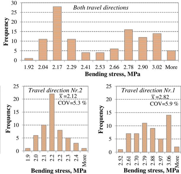
Fig. 6. Bending stresses (converted from strain measurements and decomposed by directions)
