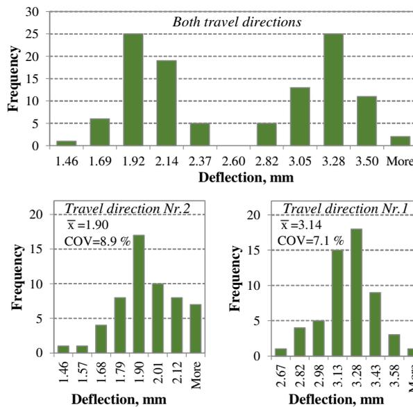
Fig. 5. Deflection measurements (decomposed by directions)
