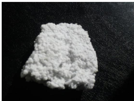
Fig. 2. **Foamed polystyrene particles are bonded with cellulose fibers**
