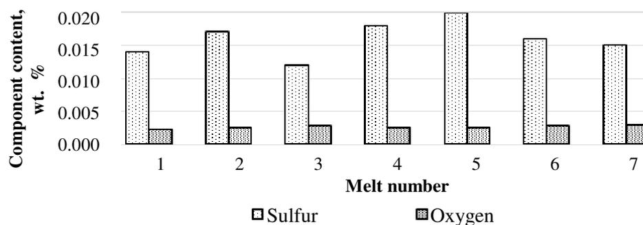
**Fig. 1. Content of sulfur and oxygen on melt numbers of steel**
