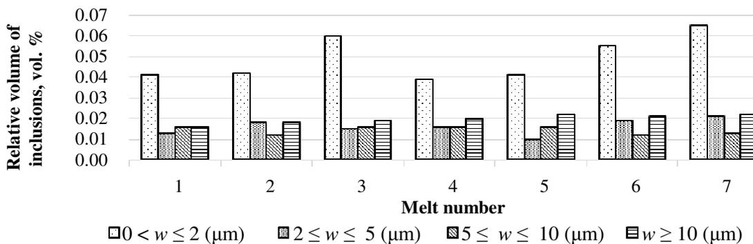
Fig. 5. Size range relative volume of inclusions on melt numbers of steel in measuring intervals
