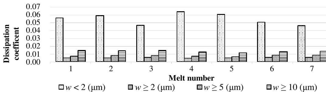
Fig. 6. Dissipation coefficient of non-metallic inclusions of steel in measuring range
