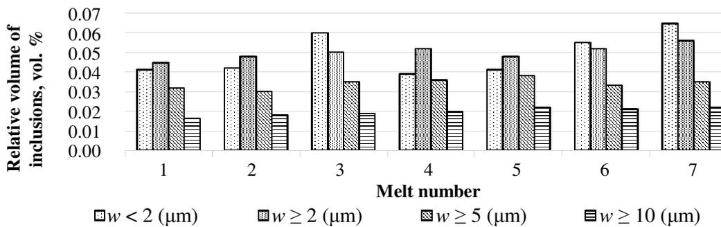
Fig. 4. Relative volume of inclusions on melt numbers of steel in size interval
