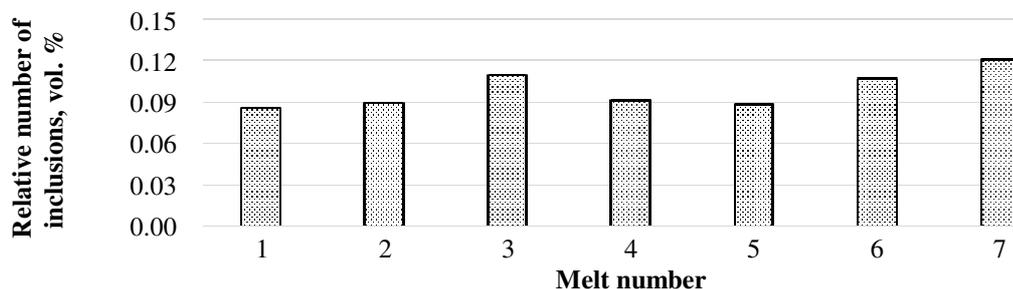
**Fig. 2. Relative volume of inclusions on melt numbers of steel**
