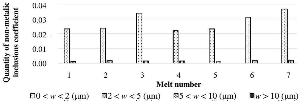
Fig. 3. Quantity of non-metallic inclusions coefficient ( $n_i$ ) in size intervals
