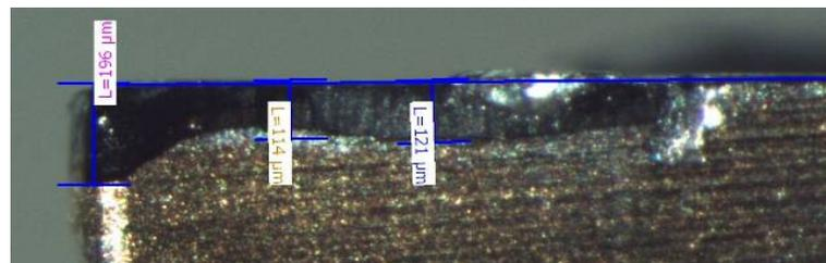
Fig. 2. Measurement of insert wear in frame of experiment with software QuickPHOTO CAMERA
