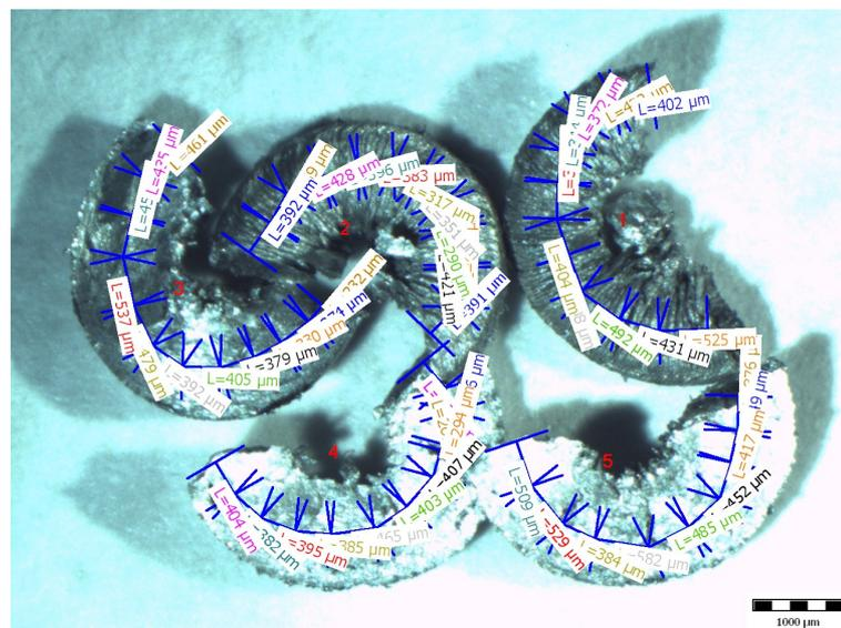
Fig. 7. Example of chip measuring
