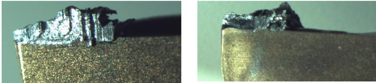
Fig. 6. Samples of created up edge (built-up) on the insert after cutting of the mentioned alloys
