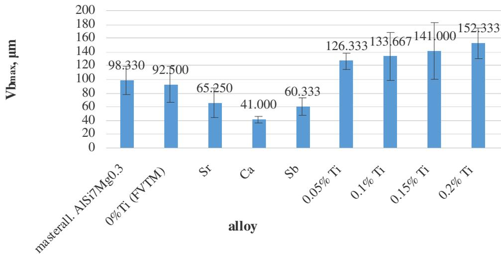
Fig. 4. Average wear VBmax for each alloy
