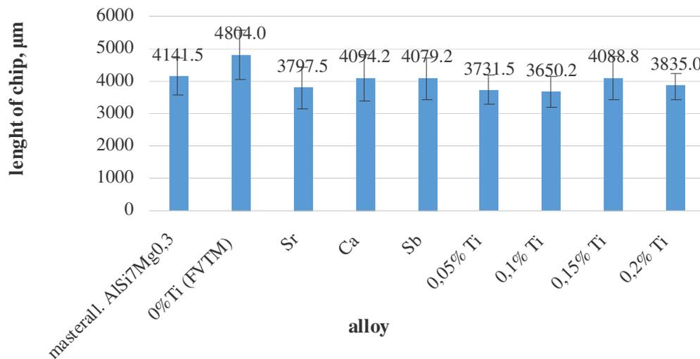
Fig. 8. Comparison of the lengths of the chips for each alloy
