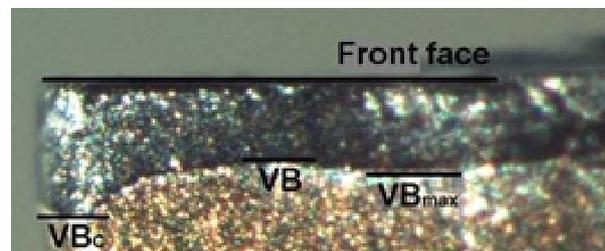
Fig. 1. Principle of measurement of wear values of cutting plate (insert)
