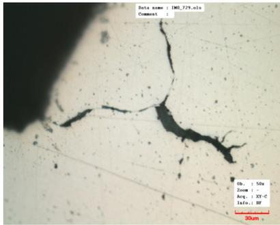
Fig. 12. Oxide membranes, inclusions
