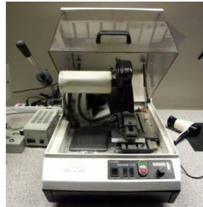
Fig. 3. Metallographic saw MTH Mikron 110
