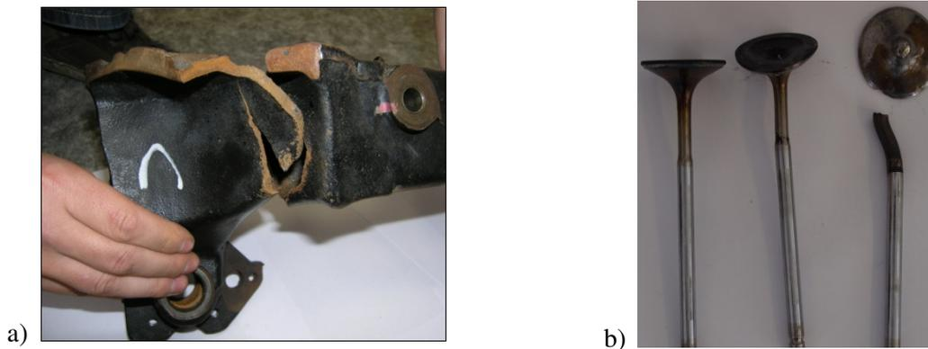
Fig. 9. Examples of the analysed components: a – part of the car chassis, fracture; b – valves, creep
