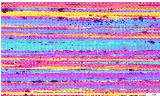
Fig. 6. Fibrous structure in the direction of forming under polarized filtered light, 600x
