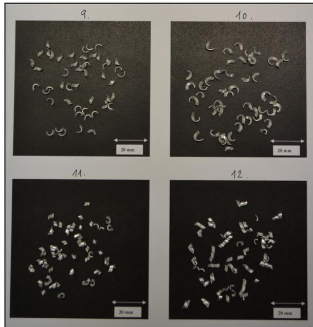
Fig. 9 Samples of preparation for evaluation of chips in terms of shapes for the selected alloys
