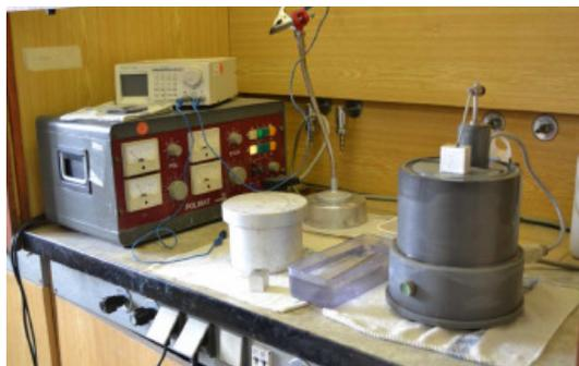
Fig. 3. Electrolytic polisher SDP 2405
