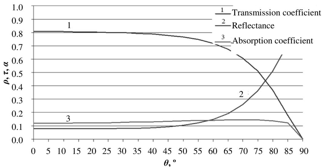
Fig. 3. Results of the calculations of reflectance  $\rho_p$ , absorption  $\alpha_p$  and transmission  $\tau_p$  coefficients
