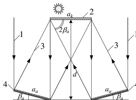
Fig. 1. **Principal scheme of solar collector with reflectors:** 1 – falling sun rays; 2 – box type absorber; 3 –reflected sun rays; 4 –reflectors
