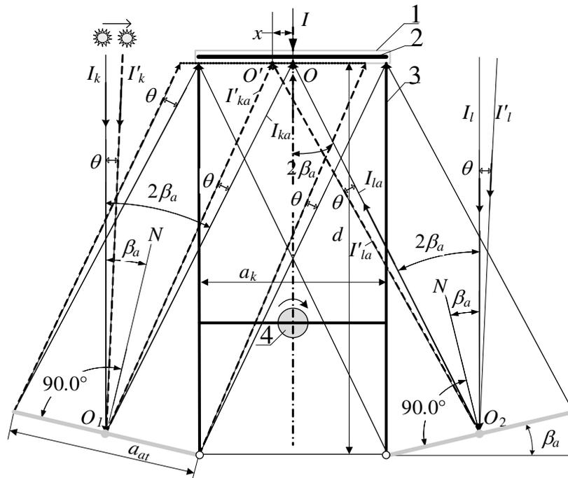
Fig. 5. **Principal scheme of operations for the solar collector with reflectors:** 1 – solar energy collector irradiated from both sides; 2 – absorber; 3 – frame; 4 – rotation mechanism
