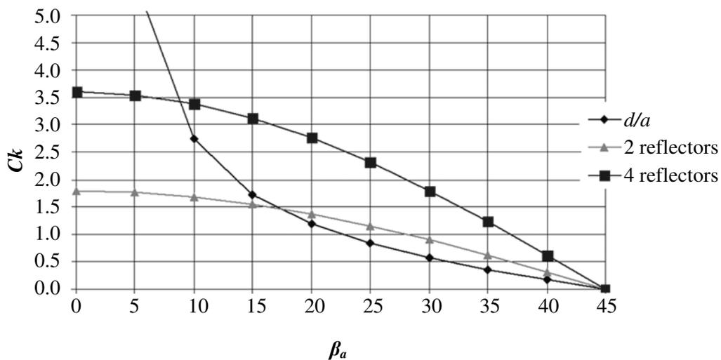
Fig. 2. Characteristics of the solar collector with reflectors:  $C_k$  – concentration ratio of reflectors;  $\beta_a$  – rotation angle of the reflectors;  $d/a$  – ratio between the distance of the reflector and the width of the solar collector
