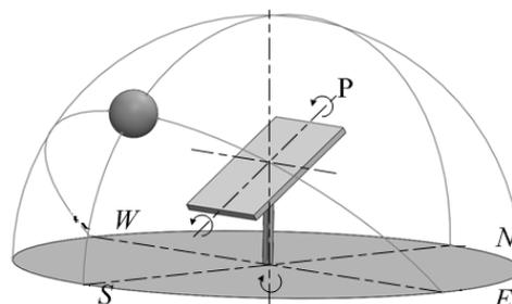
Fig. 4. Principal scheme for full tracking system
