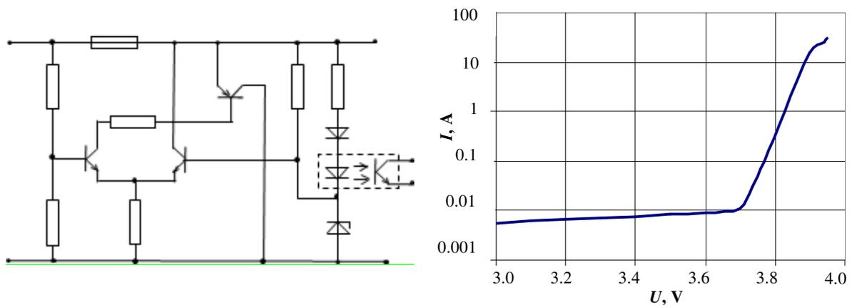
Fig. 8. Circuit diagram of the balancer and its volt -ampere characteristic
