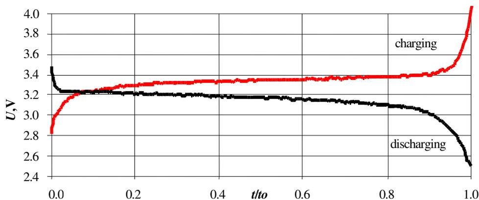
Fig. 1. LiFePO<sub>4</sub> accumulator charge/discharge curve
