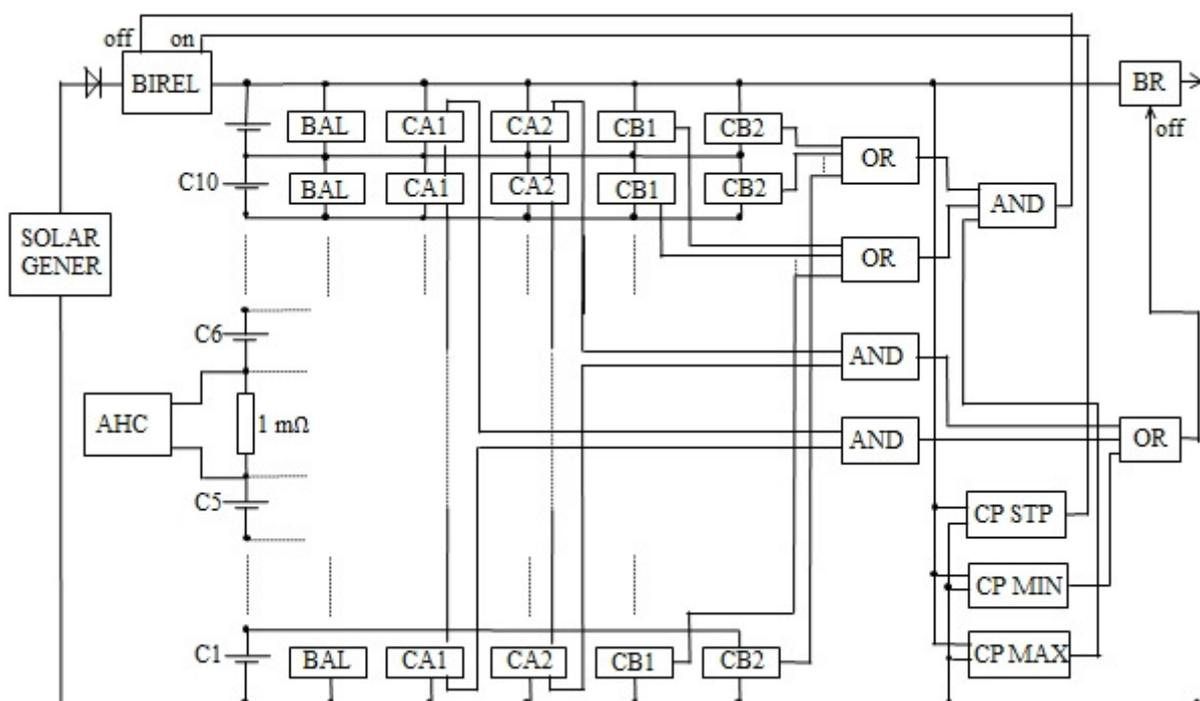
Fig. 5. Schematic block diagram of the system: AHC – amper hour counter; BAL – balancer; BIREL – bistable relays; BR – breaker;  $C_i$  ( $i = 1$  up to 11) cells; CA1, CA2 – minimal cell voltage sensors; CB1, CB2 – maximal cell voltage sensors; CP STP – comparator stop; CP MIN – comparator minimum; CP MAX – comparator maximum; SOLAR GENER – solar generator
