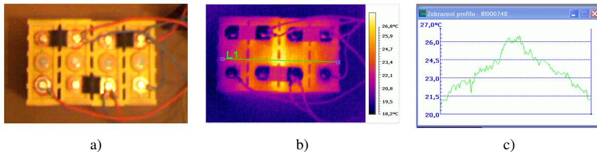
Fig. 2. **Temperature field on the accumulator:** a) photo; b) IR imag; c) temperature profile
