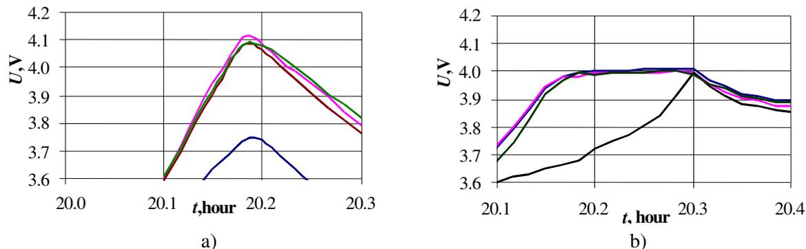
Fig. 3. **Voltages of four cells at the end of the charge cycle:** a) without balancer; b) with balancer
