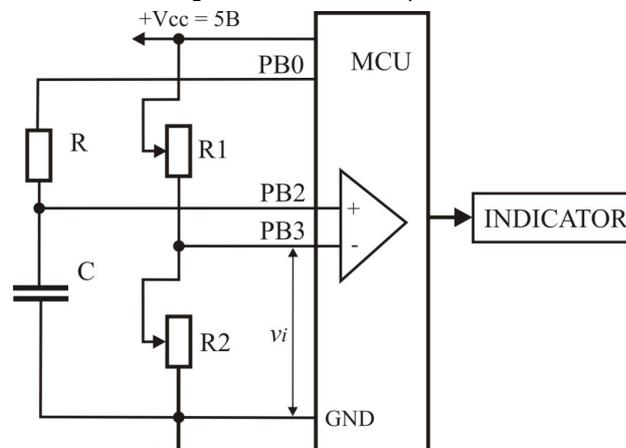
Fig. 4. Functional scheme of the device for RC-ADC study
