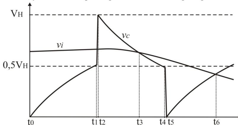
Fig. 3. Operation of RC-ADC, Timing Diagram
