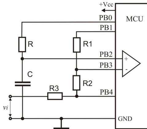
Fig. 2. Functional scheme of RC-ADC-based Microcontroller
