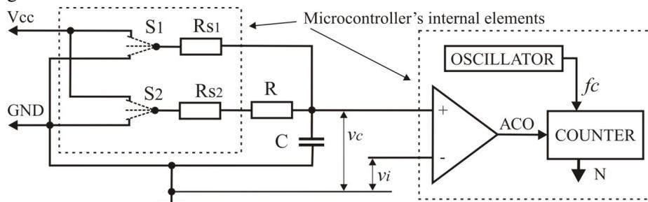
Fig. 1. Equivalent circuit of RC-ADC
