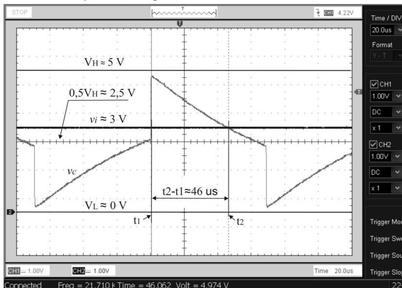
Fig. 5. Oscillogram of Capacitor voltage  $v_c$  and input voltage  $v_i$
