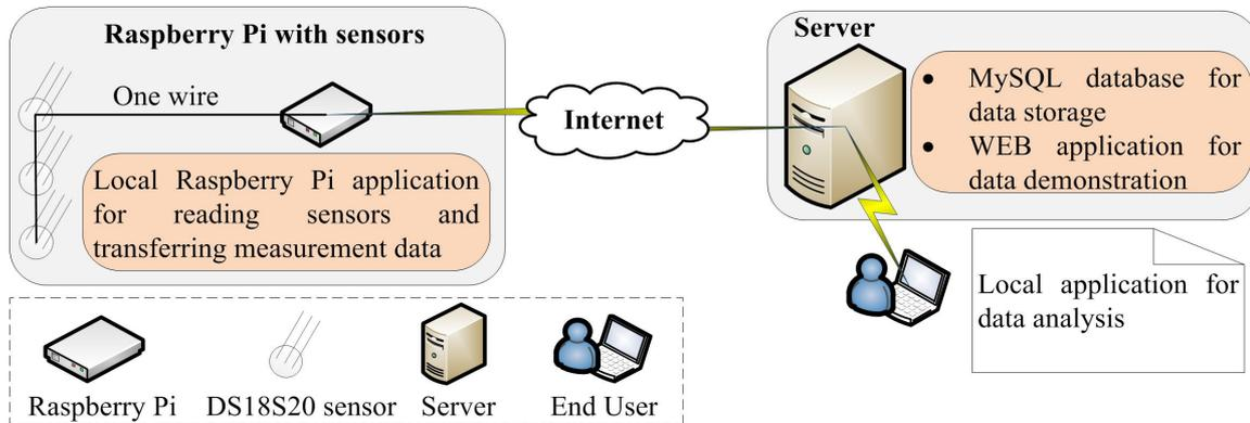
Fig. 1. System architecture used for honey bee monitoring [10]
