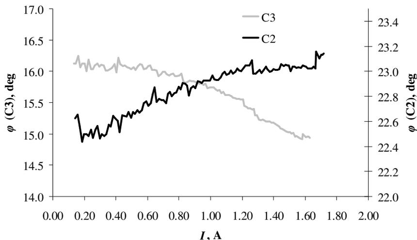
Fig. 5. Coil phase angle in relation to current (large coils)
