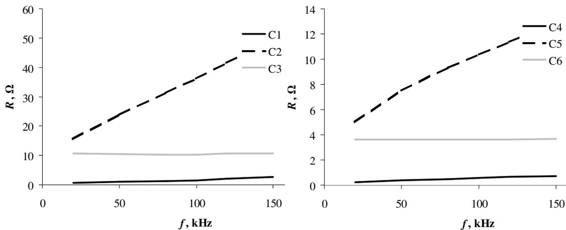
Fig. 4. Resistance  $R$  of coils in relation to frequency
