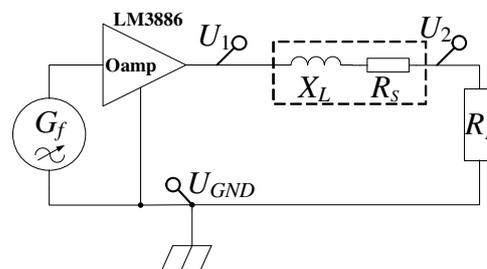
Fig. 2. Block diagram of experimental setup
