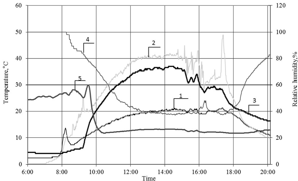
**Fig. 5. Hemp desiccation parameter characteristic graph using the heated air with the solar radiation energy concentrator:** 1 – ambient air temperature; 2 – ambient air relative humidity; 3 – outflow air temperature; 4 – temperature inside the hemp roll; 5 – relative humidity inside the hemp roll
