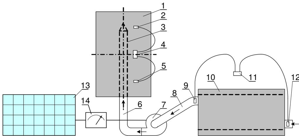
Fig. 3. **Measurement data recording scheme:** 1 – hemp roll; 2 – temperature sensor (T4); 3 – air distribution tube; 4 – data (T1;RH) recorder HOBO-H08-007-02 (Nr.853857); 5 – temperature sensor (T3); 6 – air duct; 7 – ventilator; 8 – air duct; 9 – temperature sensor (T4); 10 – two-chamber cylindrical solar air heater; 11 – data (T1;RH) recorder HOBO-H08-007-02 (Nr.697103); 12 – temperature sensor (T3); 13 – the solar cell module; 14 – voltage regulator-stabilizer
