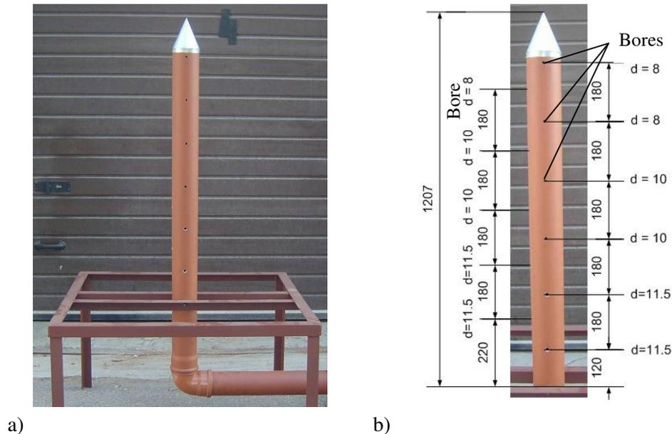
Fig. 1. Desiccation device of herbaceous plants rolled up in a roll mass:
