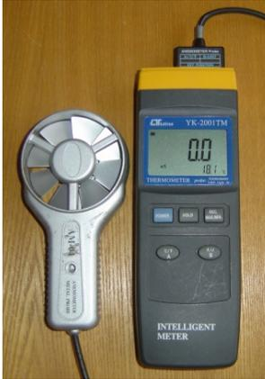
Fig. 3. Anemometer for flow measurements
