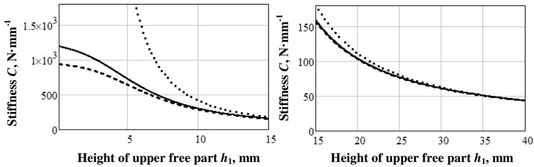
Fig. 6. Compressive stiffness dependence on height of upper free part of damper: — with friction  $f = 0.05$ ; --- neglecting friction; ···· without weak compressibility
