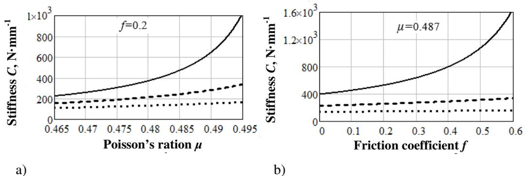
Fig. 8. Compressive stiffness dependence: a) on Poisson's ratio  $\mu$  at  $f = 0.2$ ; b) on friction coefficient  $f$  at  $\mu = 0.487$  for: —  $h_1 = 5$  mm; ---  $h_1 = 10$  mm; ····  $h_1 = 15$  mm
