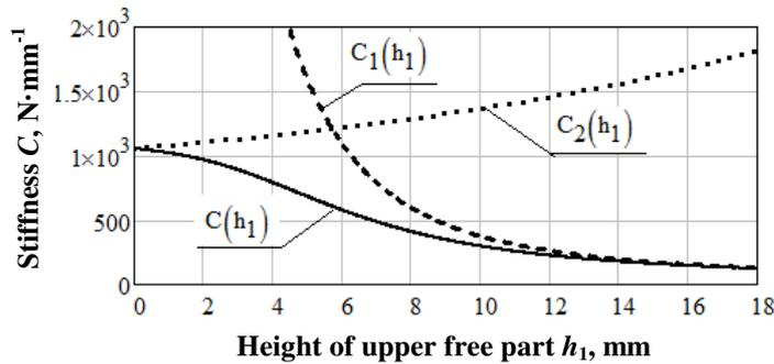
Fig. 7. Contribution of upper and lower parts to total compressive stiffness: — common stiffness  $C(h_1)$ ; --- stiffness of part 1  $C_1(h_1)$ ; ···· stiffness of part 2  $C_2(h_1)$
