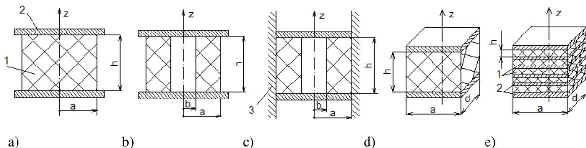
**Fig. 1. Typical elements of reinforced rubber vibroisolators operating under axial compression:**
