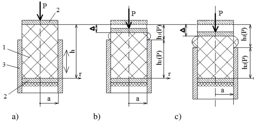
Fig. 2. **Cylindrical vibration absorber with movable cage:** 1 – elastomer; 2 – upper and lower rigid plates; 3 –movable rigid ring cage
