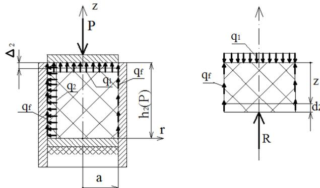
Fig. 3. **Scheme of forces acting on lower part of absorber**
