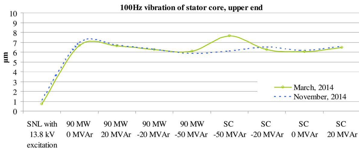
Fig. 2. Stator core vibration in different modes
