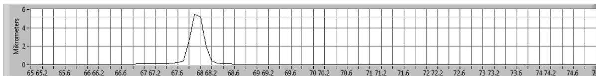
Fig. 4. 100 Hz vibration spectrum at 90 MW load with 0 MVar
