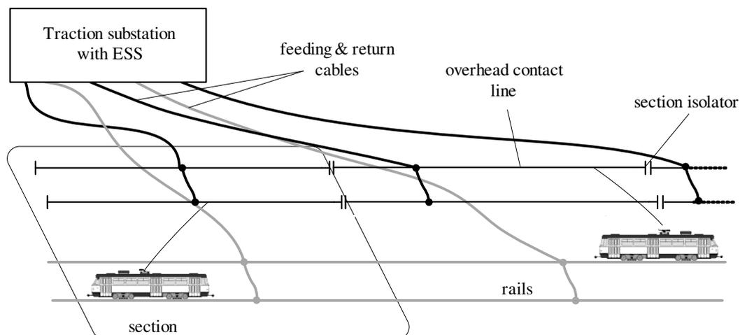
Fig. 1. Tram system with “radial topology”
