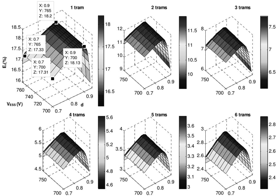
Fig. 5. ESS control parameter influence on energy consumption from substation
