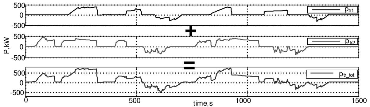
Fig. 3. Synthesis of tram power profiles
