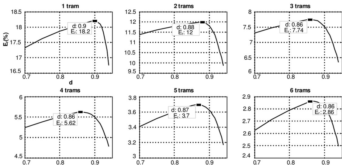
Fig. 5. ESS discharge level effect on energy consumption from substation at  $V_{ESS} = 765$  V
