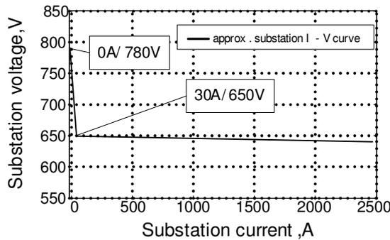
Fig. 4. I-V curve of traction substation
