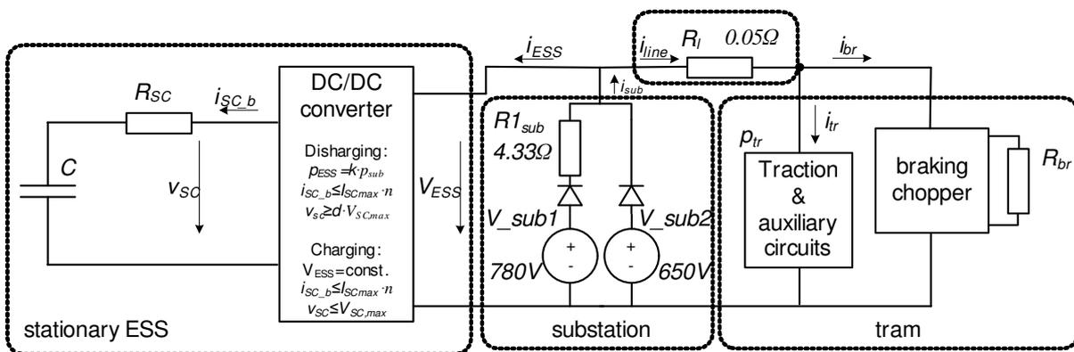
**Fig. 2. Block diagram of mathematical model for tram system with stationary ESS**
