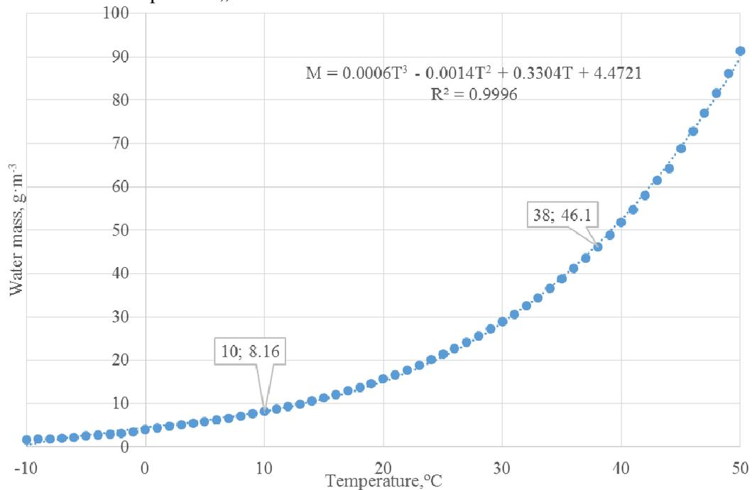
Fig. 1. Content of water in the air with different temperatures (100 % relative moisture)
