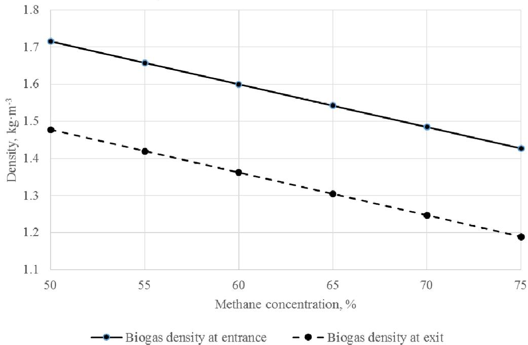
**Fig. 2 Biogas density dependence on methane concentration at dryer entrance and exit**
