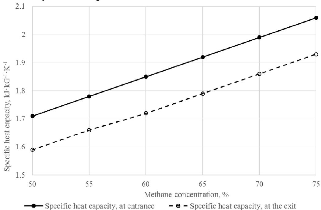
**Fig. 3 Biogas specific heat capacity dependence on methane concentration at dryer entrance and exit**
