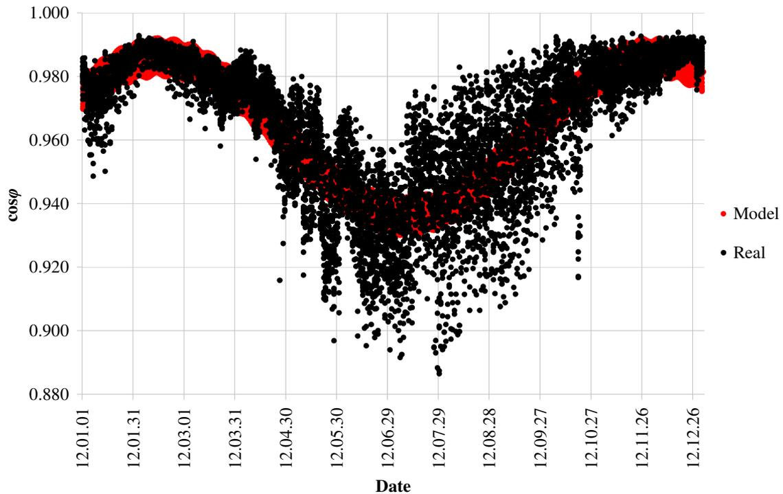
Fig. 4. Mathematic model  $\cos\phi = f(t)$  application on observed power factor data
