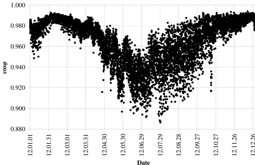
Fig. 3. Power factor  $\cos\phi = f(t)$  calculated from collected data
