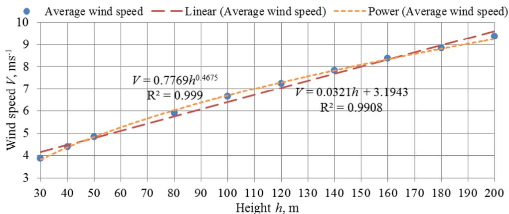
Fig. 3. Average wind speed for 03.2014-03.2015 with linear and power models
