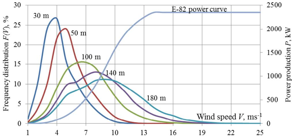
Fig. 4. Wind speed frequency distribution for period 03.2014-03.2015 with power curve of wind turbine Enercon E-82 with rated power 2300 kW
