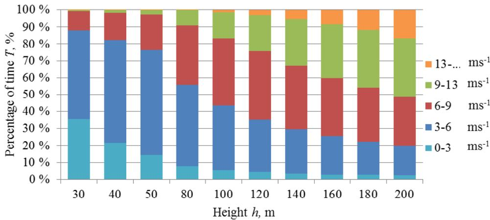
Fig. 5. Relative time duration  $T$ , % of air flow with wind speed in intervals 0-3, 3-6, 6-9, 9-13, 13-... m·s<sup>-1</sup> up to height of 200 m for one year measurement period
