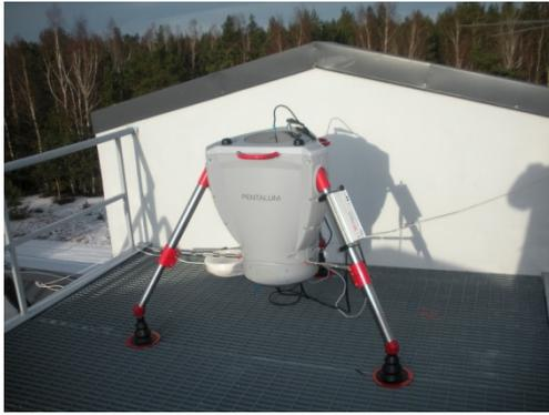
Fig. 1. Pentalum SpiDAR located in Irbene, Latvia
