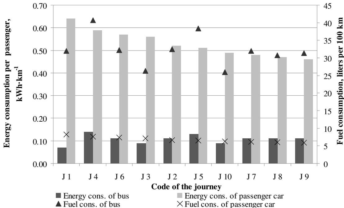
Fig. 3. Energy and fuel consumption of public transit and passenger car transport
