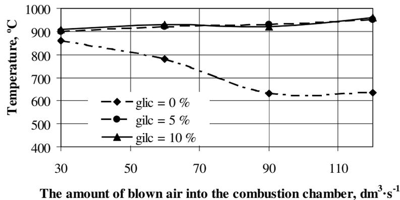
Fig. 2. Temperature in burning chamber
