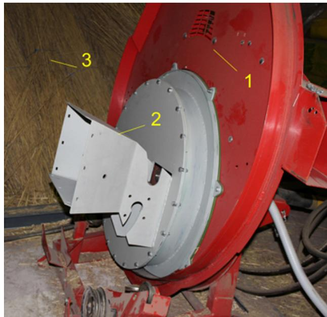
Fig. 1. **Modified bale shredder:** 1 – frame; 2 – bundle feeder mechanism; 3 – common reed bundles
