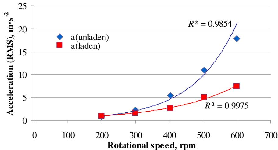
Fig. 4. Cutter head bearing housing vibration acceleration (RMS) values
