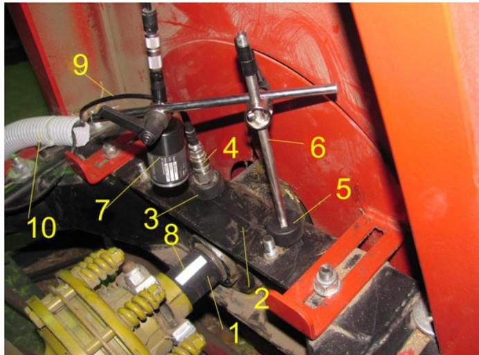
Fig. 2. Vibration sensor montage on bearing housing
