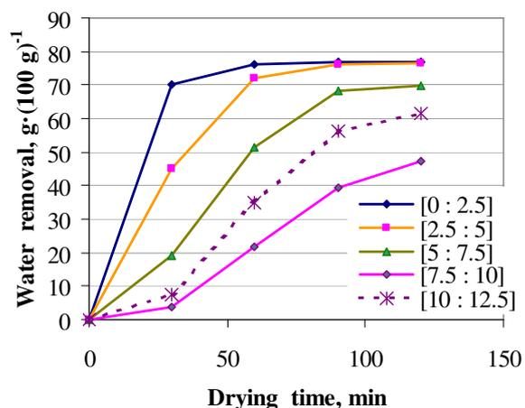
Fig. 5. Average amount of water removal from beer dregs layers by venting with temperature 52 °C
