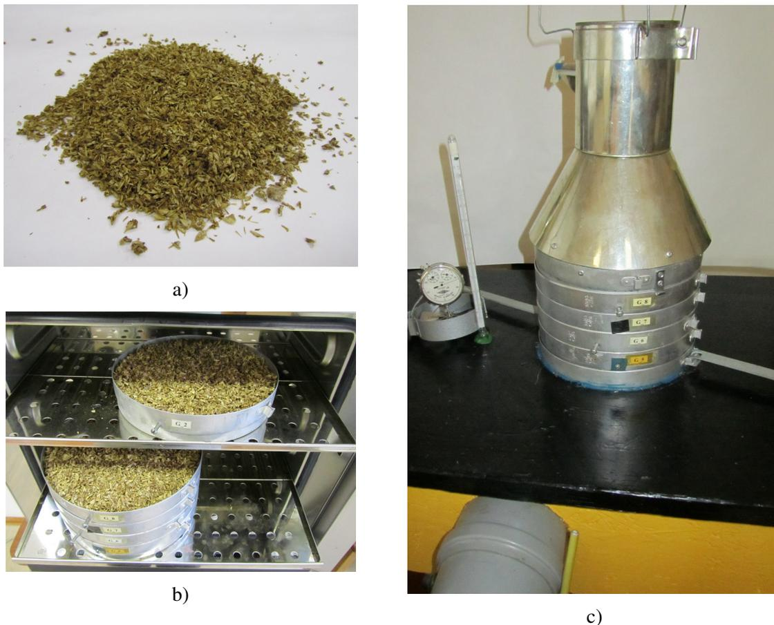
Fig. 1. **Material and experimental equipment:** a) dried beer dregs, b) cassettes with beer dregs in drying cabinet “EMMERT”, c) beer dregs drying by ventilation
