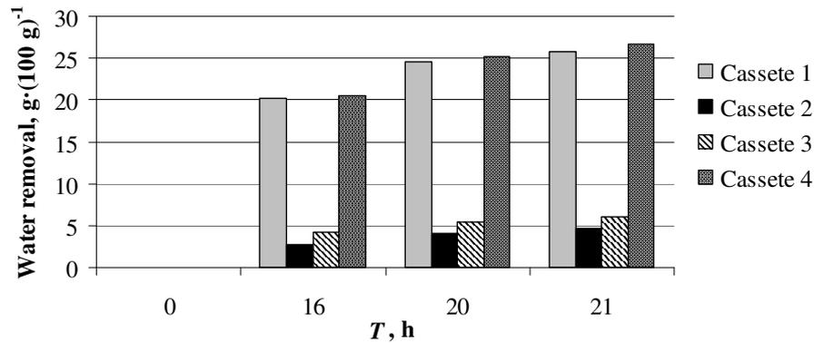
Fig. 2. Average moisture removal from 4 cassettes in 10 cm thick layer depending on the drying time  $T$
