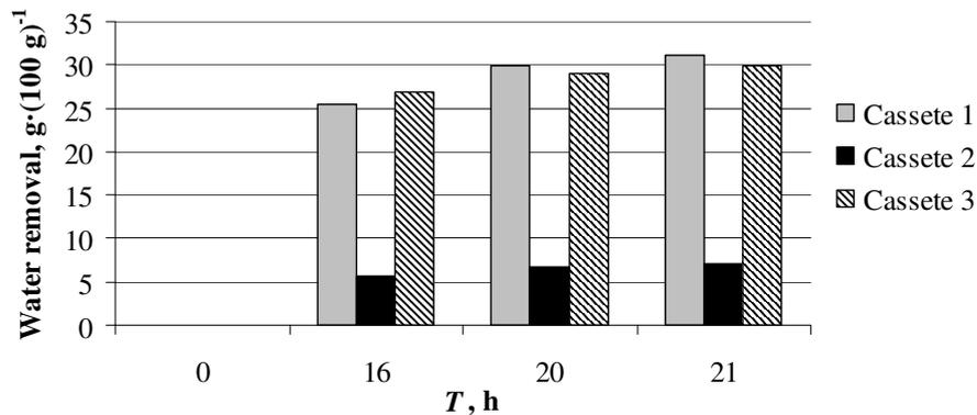
Fig. 3. Average moisture removal from 3 cassettes in 7.5 cm thick layer depending on the drying time  $T$
