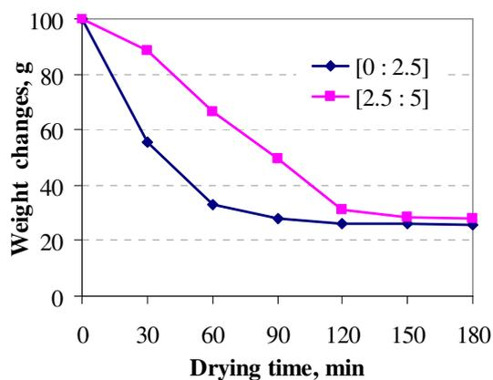
Fig. 4. Beer dregs layers weight changes during venting with temperature 35 °C
