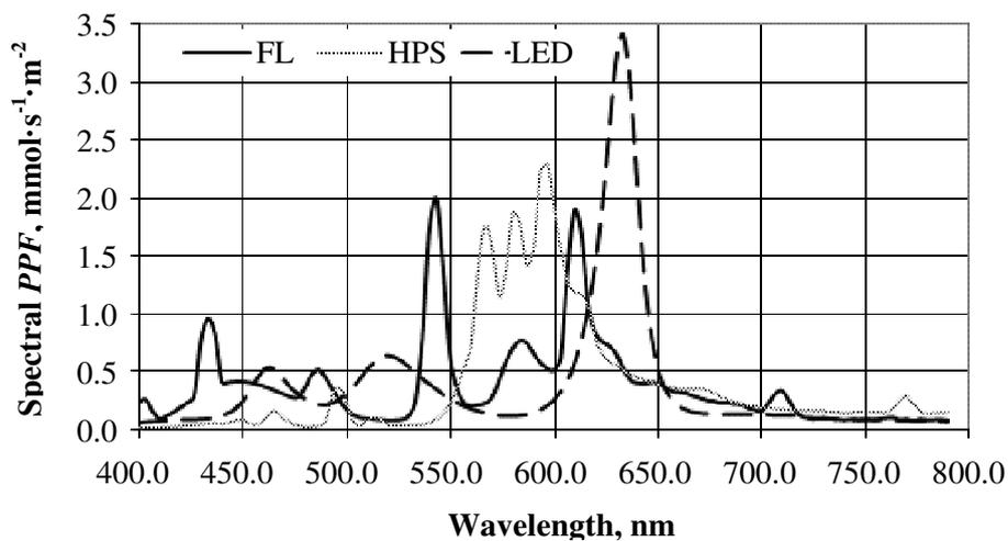
Fig. 2. Spectrum density of PPF
