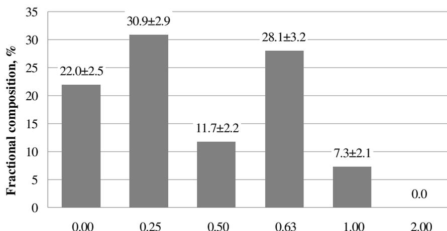
Fig. 2. Fraction composition of oak leaves mill (diameter of holes in mm)
