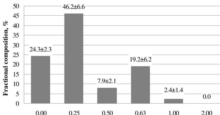
**Fig. 1. Fraction composition of oak bark mill (diameter of holes in mm)**
