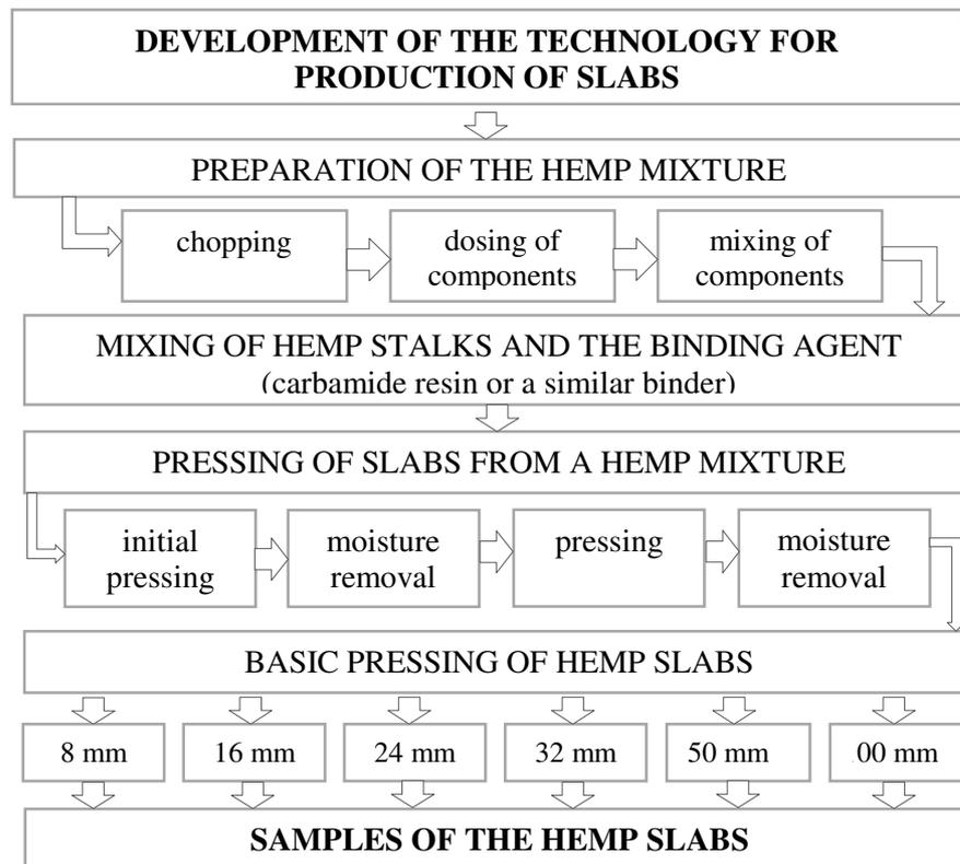
Fig.1. Scheme of the slab production technology
