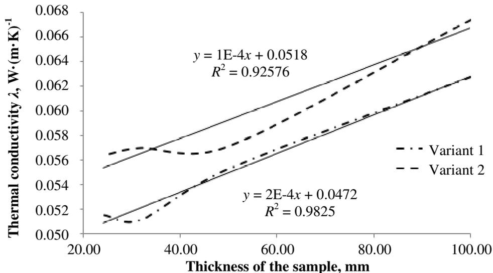
Fig. 8. Thermal conductivity of a slab depending on its thickness
