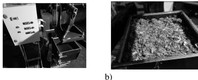
Fig. 5. Press for pressing the fleece material: a – pressing equipment; b – pressing chamber
