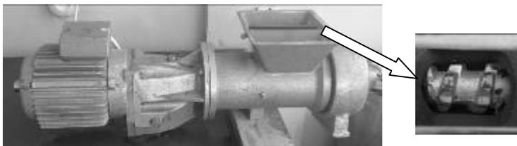
Fig. 3. **Extruder for disintegration of the hemp mass**
