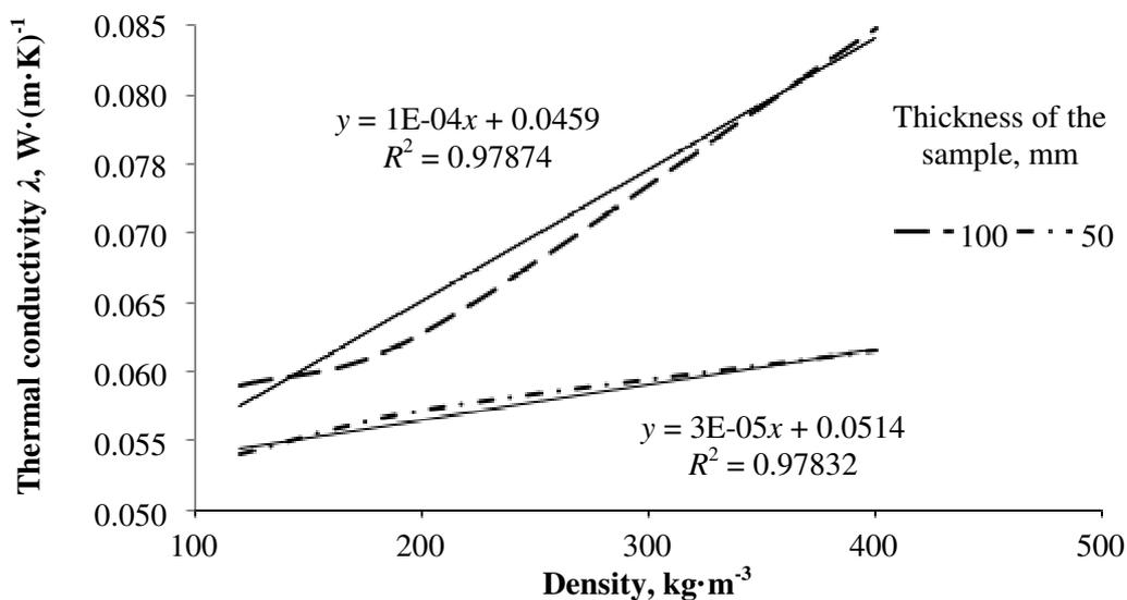
Fig. 7. Thermal conductivity of a slab depending on its density
