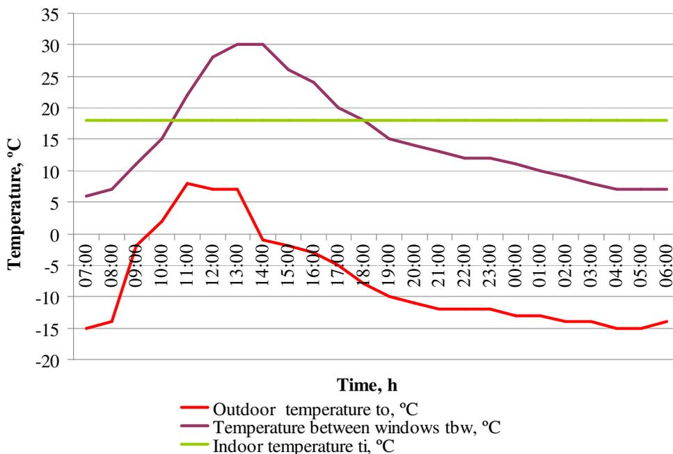
Fig. 3. Example of temperature changes in air gap (Fig. 1) during 24 hours (17<sup>th</sup> Jan 2015)
