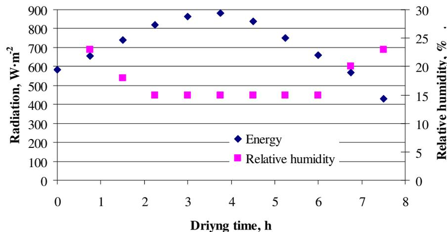
Fig. 4. Dependency between solar radiation and humidity drying time
