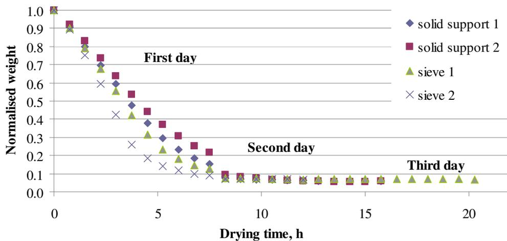
Fig. 3. Dependency between normalised weight and drying time without night time
