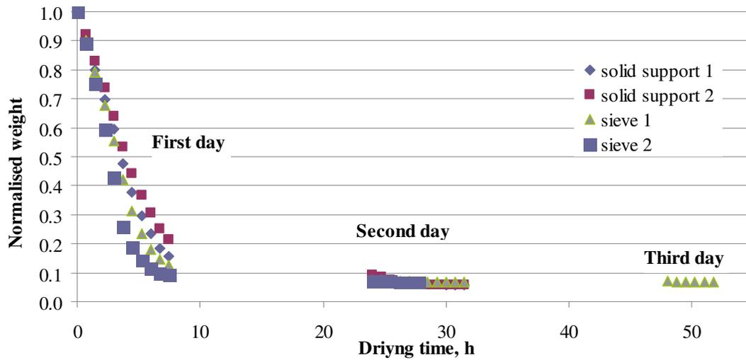
Fig. 2. Dependency between normalised weight and drying time
