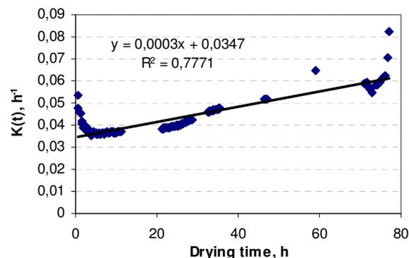
Fig. 3. Linear drying rate  $K(t)$  calculation for pine cone drying placed on sieve
