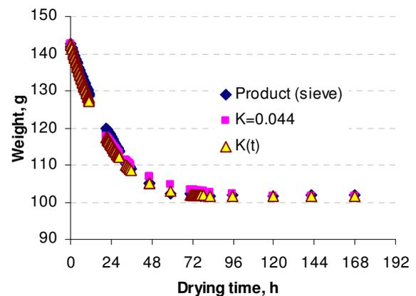
Fig. 5. Pine cone weight change (experimental and theoretical calculated) during drying on a sieve
