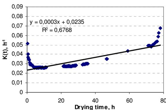
Fig. 2. Linear drying rate  $K(t)$  calculation for pine cone drying placed in bowl
