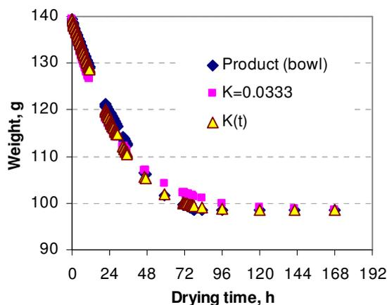
Fig. 4. Pine cone weight change (experimental and theoretical calculated) during drying in a bowl
