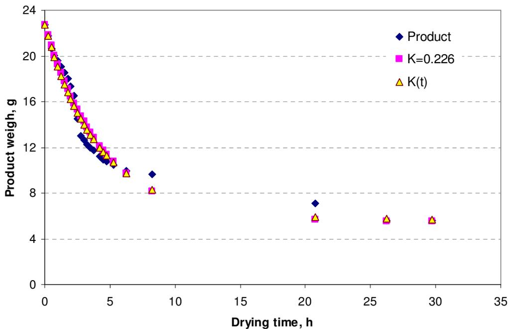
Fig. 7. Peppermint (*Mentha piperita* L.) plant weight change (experimental and theoretical calculated) during drying on a white bowl
