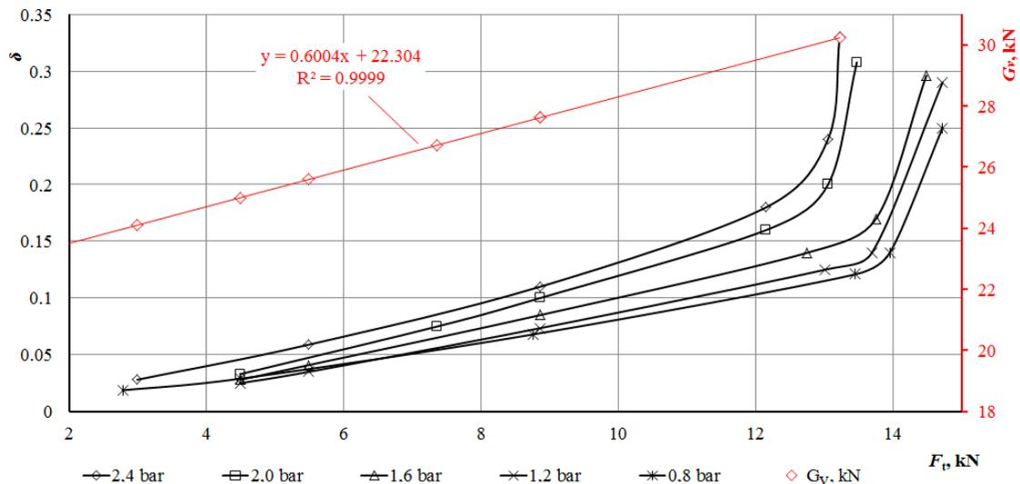
**Fig. 3. Dependence of the rear wheel coefficient of slippage  $\delta$  on different inflation pressure in the rear tires of drawbar pull  $F_t$  driving the tractor “New Holland T5070” in the stubble, when the inflation pressure in the rear tires: 0.8; 1.2; 1.6; 2.0, 2.4 bar; vertical load of the rear wheels  $G_v$  dependence of drawbar pull  $F_t$**
