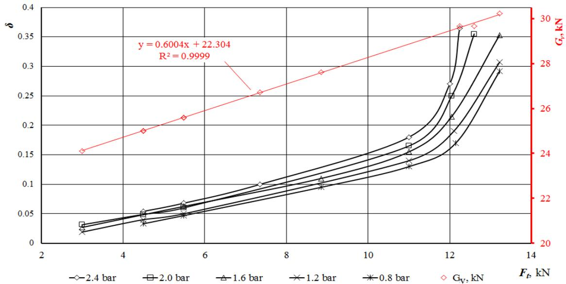
**Fig. 2. Dependence of the rear wheel coefficient of slippage  $\delta$  on different inflation pressure in the rear tires of drawbar pull  $F_t$  driving the tractor “New Holland T5070” in the soil preparing for sowing, when the inflation pressure in the rear tires: 0.8; 1.2; 1.6; 2.0, 2.4 bar. Vertical load of the rear wheels  $G_v$  dependence on drawbar pull  $F_t$**
