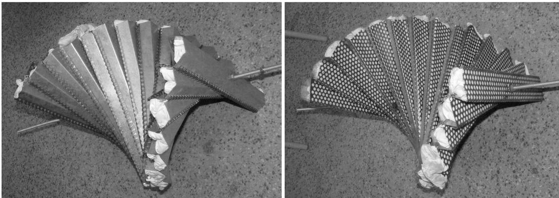
Fig. 2. Special spiral silencer before installation into the air-duct:
