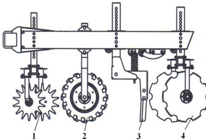
Fig. 1. **Strip-tillage equipment:** 1 – row cleaners, 2 – supporting wheel, 3 – coulter, 4 – discs
