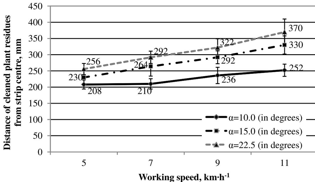
Fig. 3. Working speed and row cleaner attack angle influence on the cleaned off crop residues distance from the centre of the strip, where  $L = 105 \text{ mm}$
