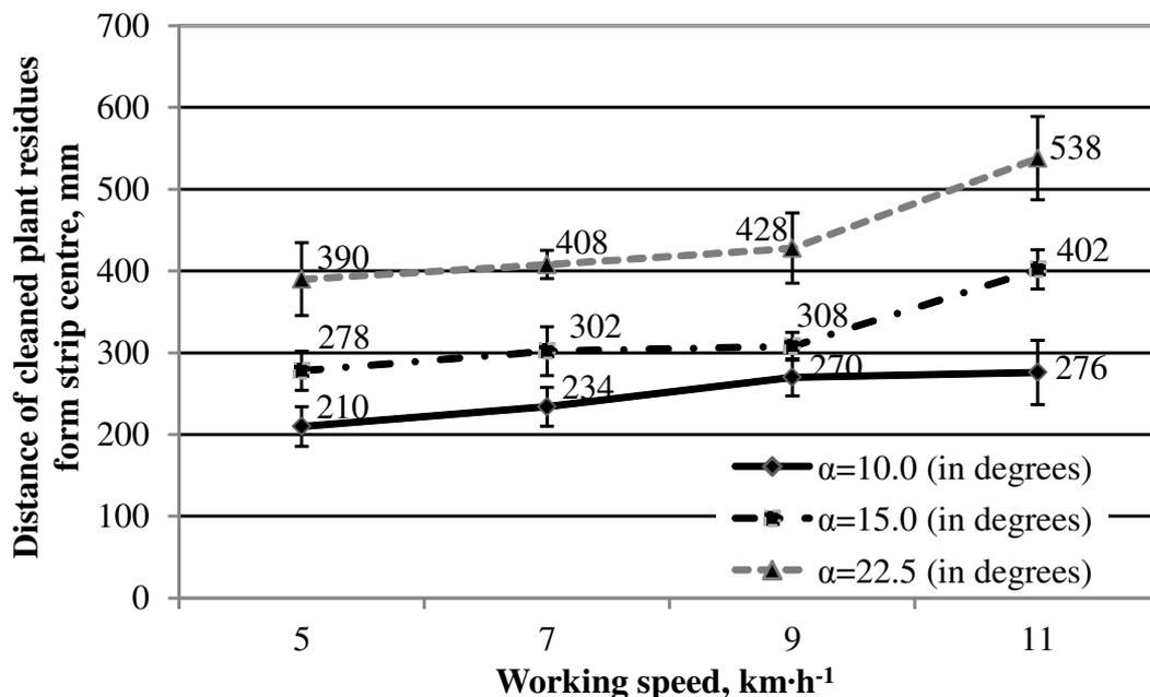
Fig. 4. Working speed and row cleaner attack angle influence on the cleaned off crop residues distance from the centre of the strip, where  $L = 120 \text{ mm}$
