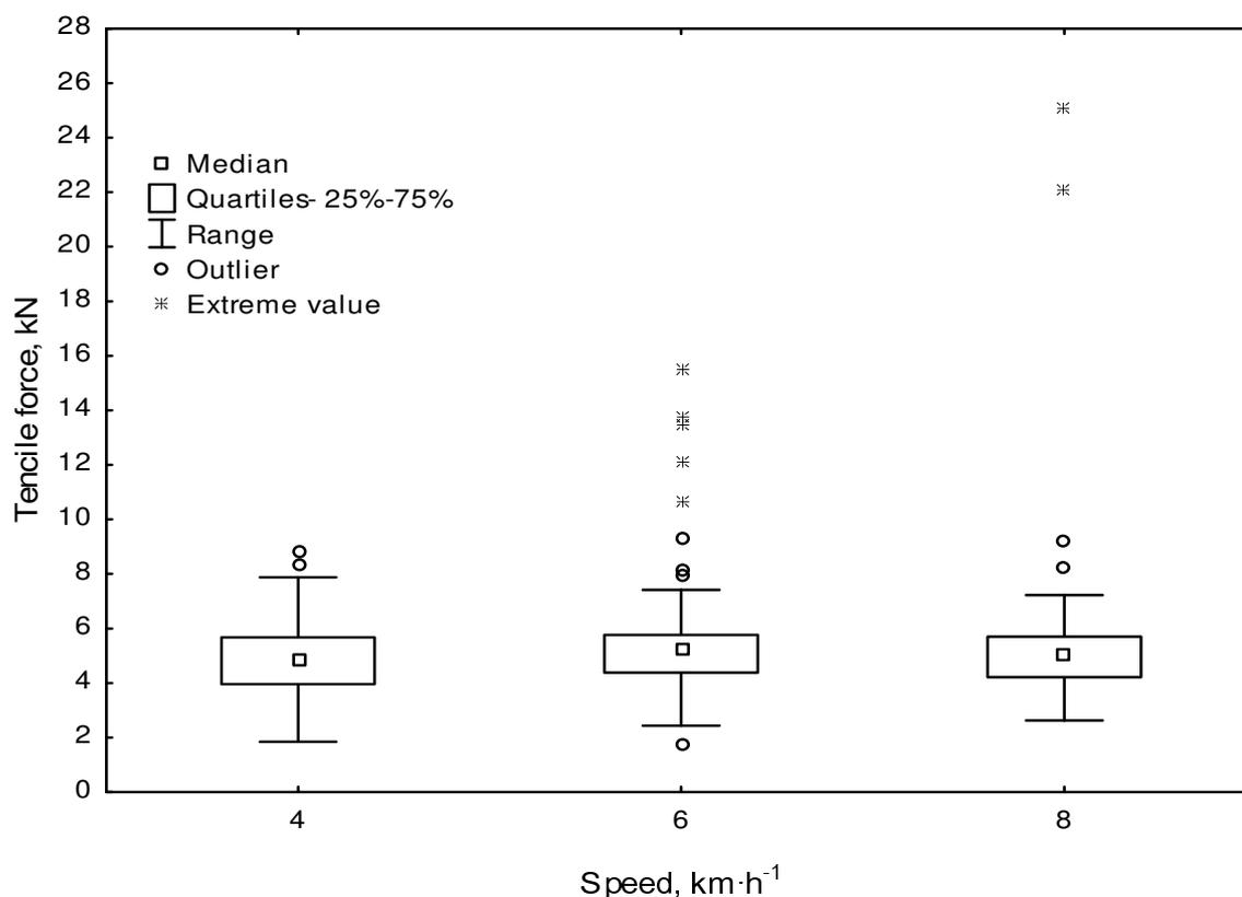
Fig. 5. Dependence of tensile force on pulling speed
