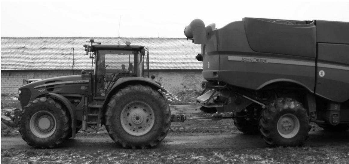
Fig. 2. Measuring set, from left: pulling tractor John Deere 7930, measuring instrument, pulled combine harvester John Deere S690i without header
