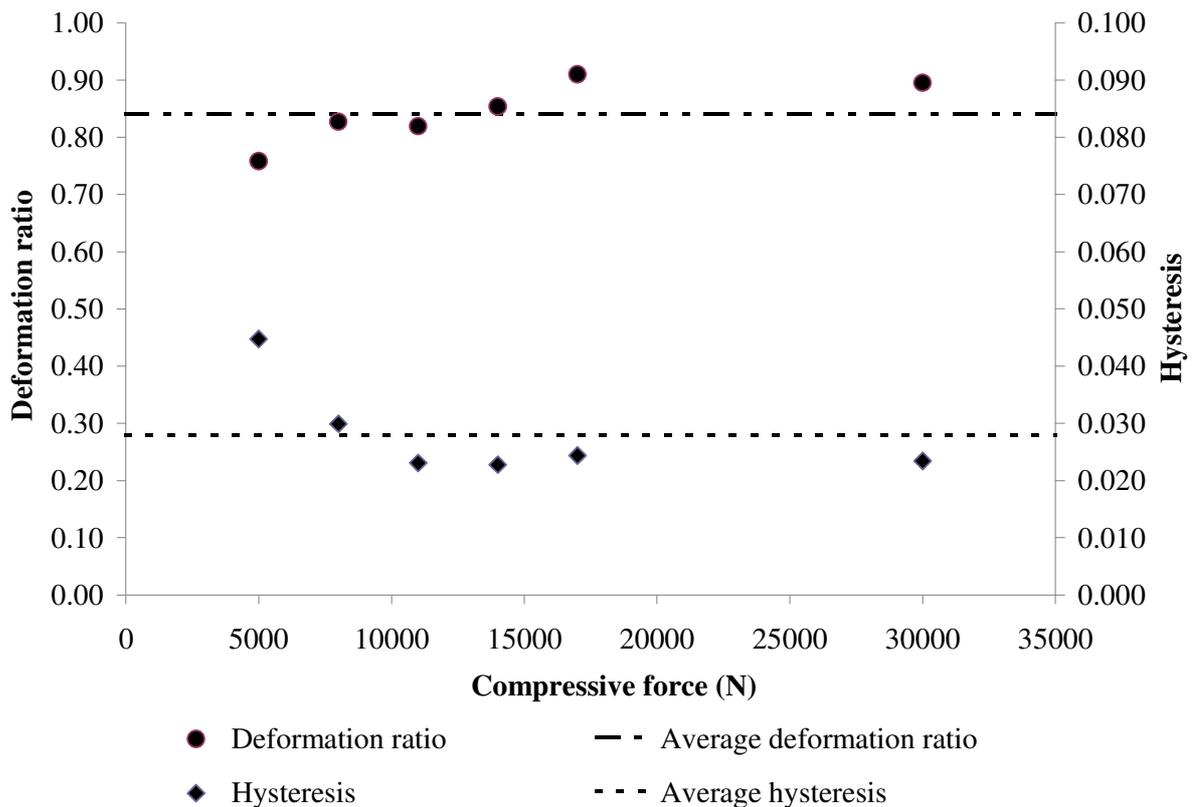
Fig. 3. Dependency of deformation ratio and hysteresis versus compressive force
