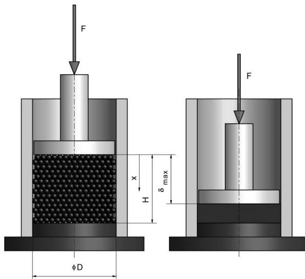
Fig. 1a. Scheme of pressing equipment
