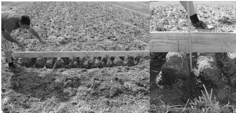
Fig. 1. Furrow bottom profile measurement
