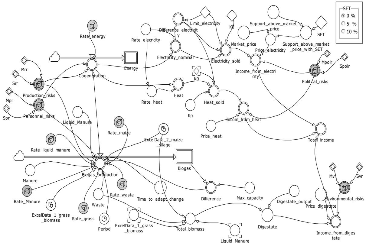
Fig. 3. Flow diagram for the dynamic model in biogas production
