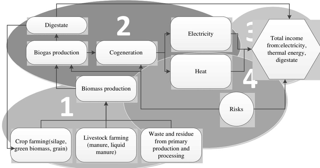
**Fig. 2. Structural scheme of the model for biogas production from agricultural biomass**
