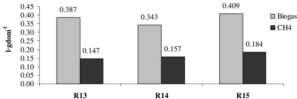
Fig. 4. Biogas and methane l·g<sub>dom</sub><sup>-1</sup> from osier (*Salix viminalis* L.)
