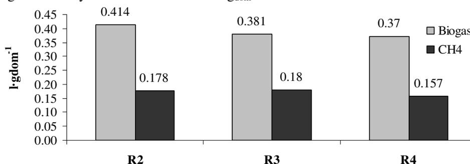
Fig. 1. Biogas and methane l·g<sub>dom</sub><sup>-1</sup> from willow Ingers
