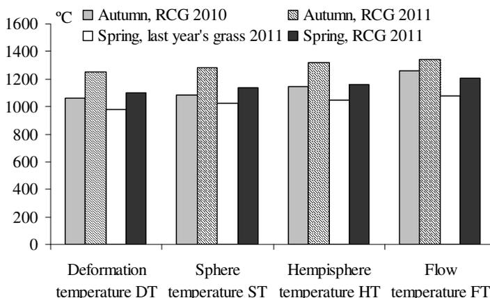
Fig. 3. Ash melting temperatures of last year's grass and RCG biomass
