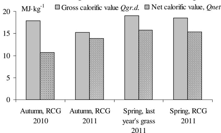
Fig. 2. Calorific value of spring last year's grass and RCG
