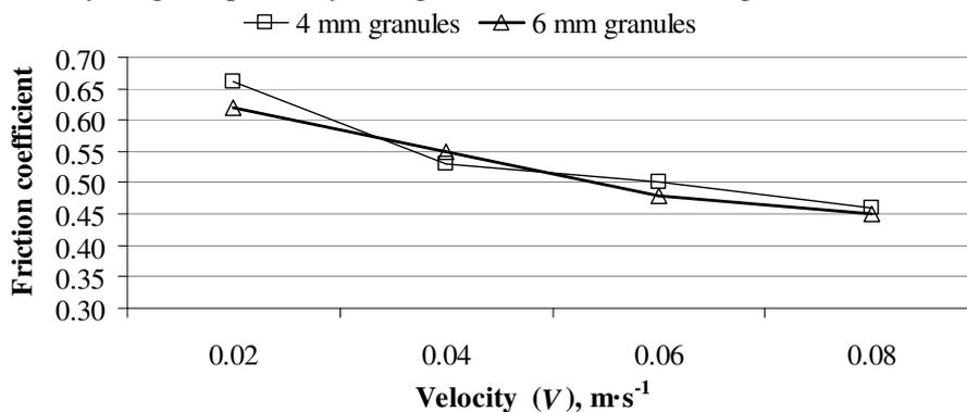
Fig. 4. Dependence of the granule dynamic friction coefficient ( $f_i$ ) on the velocity (V), when the friction surface is steel
