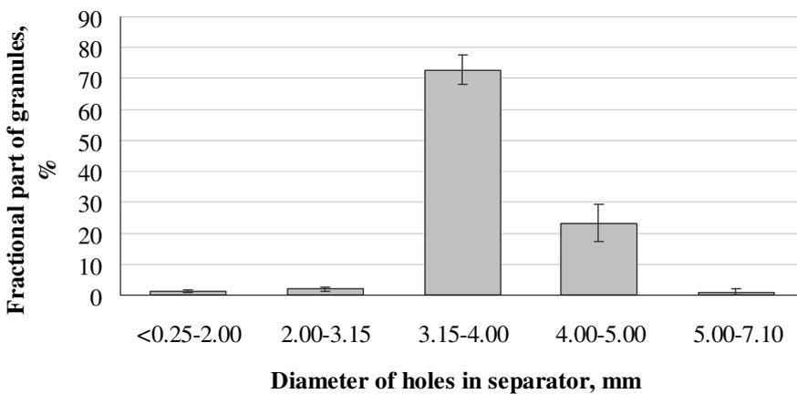
Fig. 3. Fraction part (%) of granules (diameter - 4 mm) dependence on separator holes diameter (mm)
