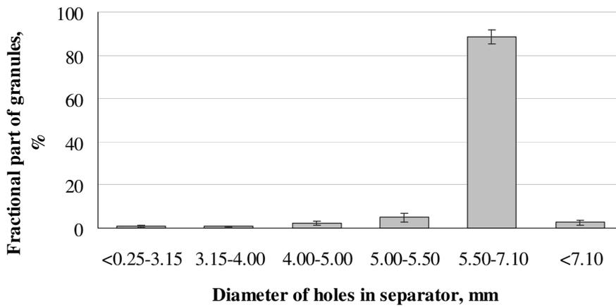
Fig. 2. Fraction part (%) of granules (diameter – 6 mm) dependence on separator holes diameter (mm)
