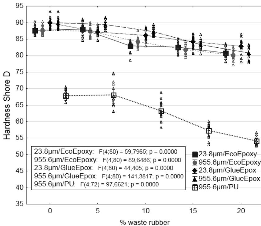
Fig. 3. Hardness Shore D of filled systems
