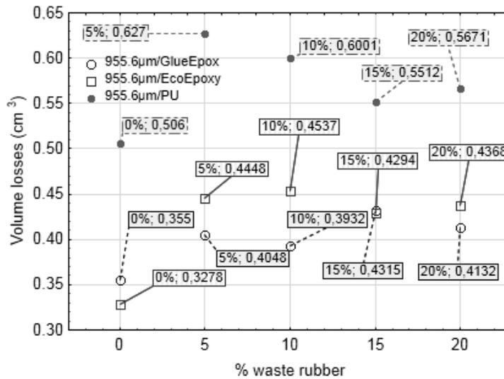
Fig. 4. Resistance to abrasive wear – particles 955.6 µm
