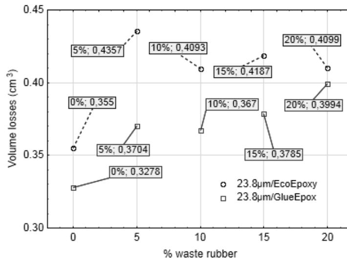
Fig. 5. Resistance to abrasive wear – particles 23.8 µm
