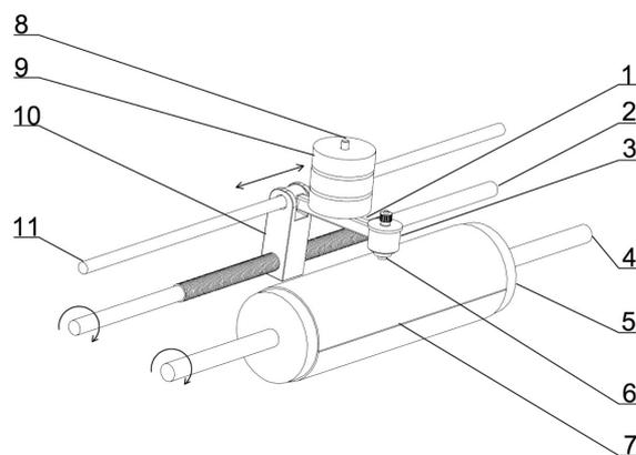
Fig. 1. **Schema of equipment for abrasive wear testing:** 1 – handle; 2 – screw; 3 – head; 4 – abor; 5 – cylinder; 6 – test sample; 7 – abrasive cloth; 8 – holder; 9 – weight; 10 – nut; 11 – rod
