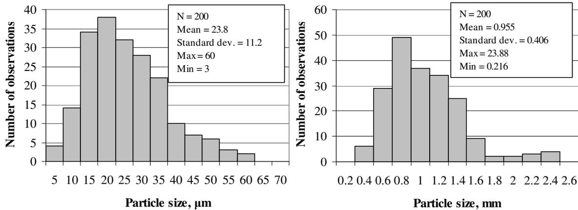
Fig. 2. Histograms of particle size 23.8 µm (left), 955.6 µm (right)
