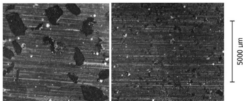
Fig. 6. Surface of materials after wearing – GlueEpoxy 10 %: 955.6 µm – left, 23.8 µm – right
