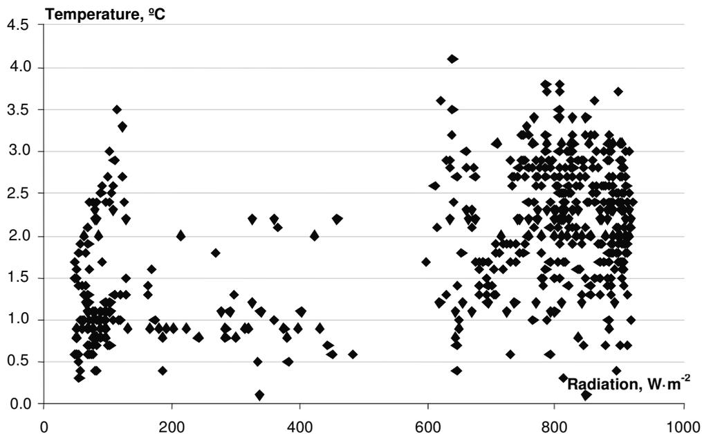
Fig. 4. Outlet air temperature from collector with water radiator and without radiator difference depending on solar radiation (9:30-19:00 14.06.2012)
