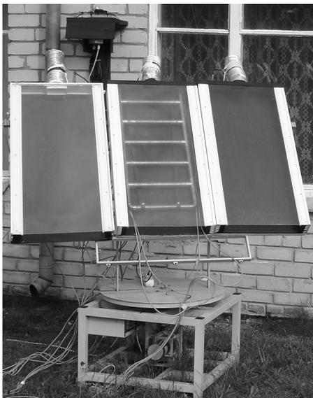
Fig. 1. View of the air heating solar collectors during the experiment
