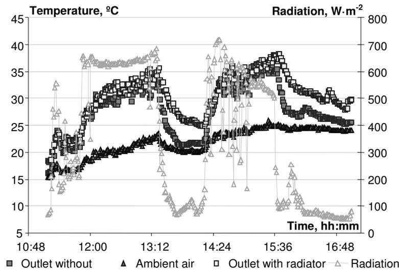
**Fig. 5. Outlet air temperatures from collector with water radiator and without radiator comparing with solar radiation and ambient temperature (11:00-17:10 11.09.2012)**
