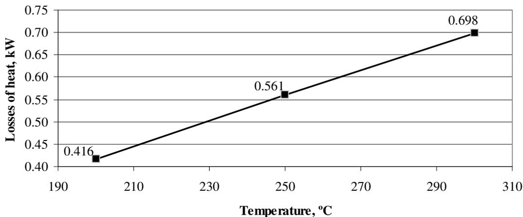
Fig. 2. Diagram for determination of the losses of heat in the equipment depending on the regulated (rated) temperature inside the heating unit
