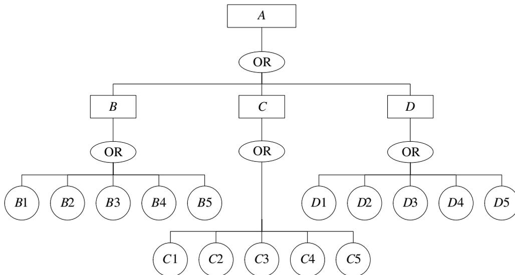
**Fig. 2. Reliability block diagram of casual events, affecting operation of packing line (initial model)**
