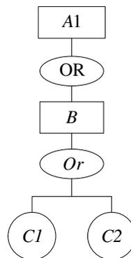
**Fig. 3. Reliability block diagram of casual events, affecting operation of packing line after improvement in performance**
