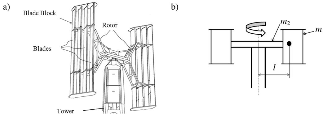
Fig. 1. **Wind turbine mechanical design according to the patent [5]:** a – full structure; b – simplified structure for calculation of the moment of inertia ( $m_1$  – blade block mass, kg;  $m_2$  – rotor mass, kg;  $l$  – radius of mass centre).
