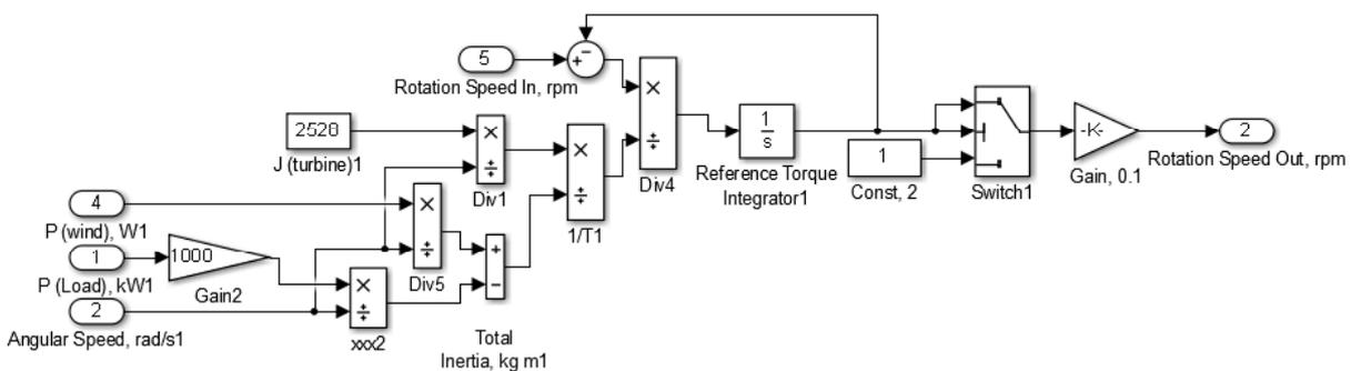
Fig. 4. Subsystem model of the wind turbine transfer process simulation
