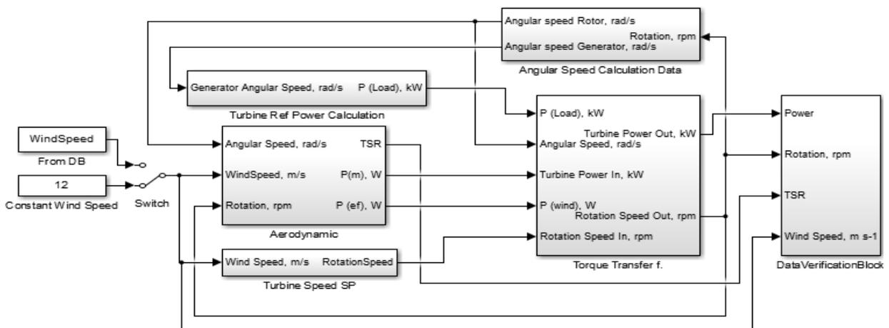
Fig. 2. Virtual model of the wind turbine in MATLAB SIMULINK
