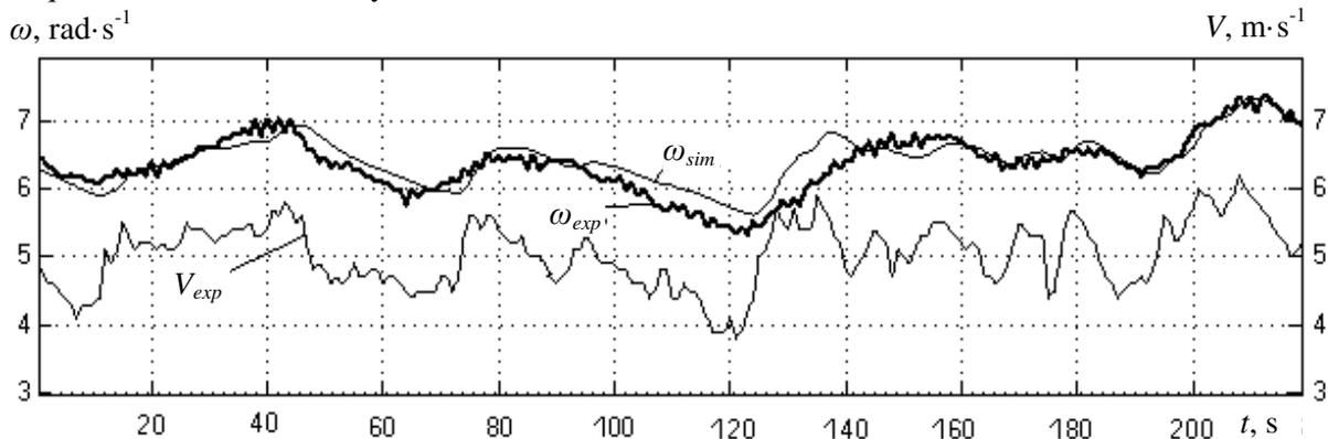
Fig. 5. Characteristic curves of the wind turbine angular speed  $\omega(t)$  and wind speed  $V(t)$ :
