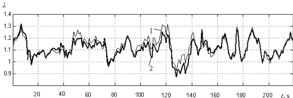
Fig.6. Characteristic curves of the wind turbine tip speed ratio  $\lambda(t)$ :
