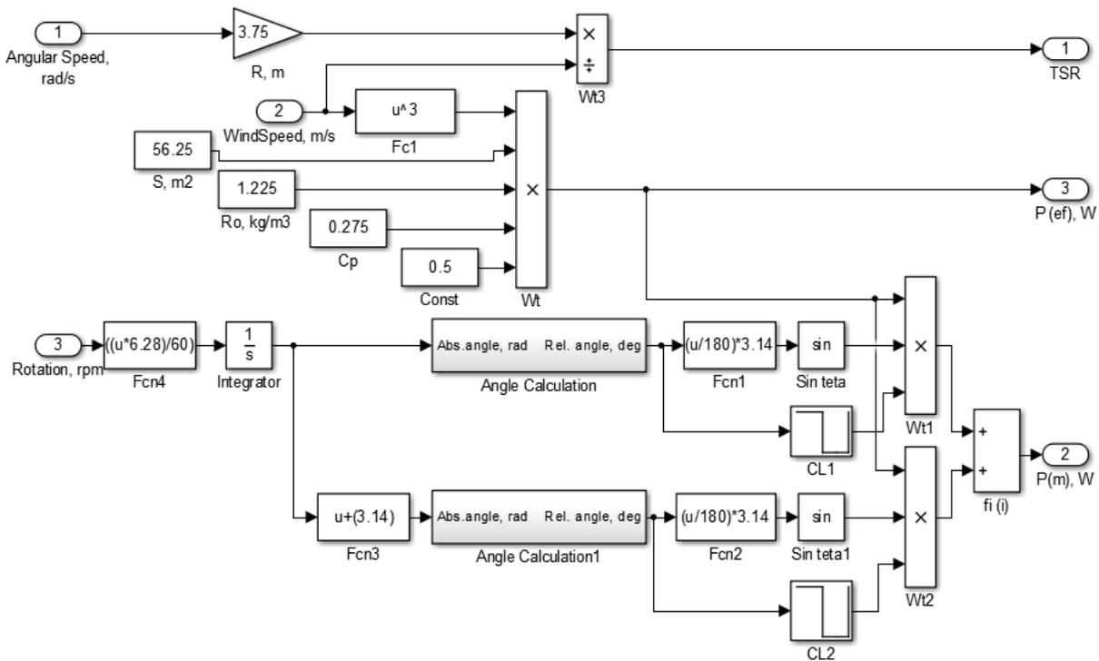
Fig. 3. Virtual model of the wind generated torque of the turbine
