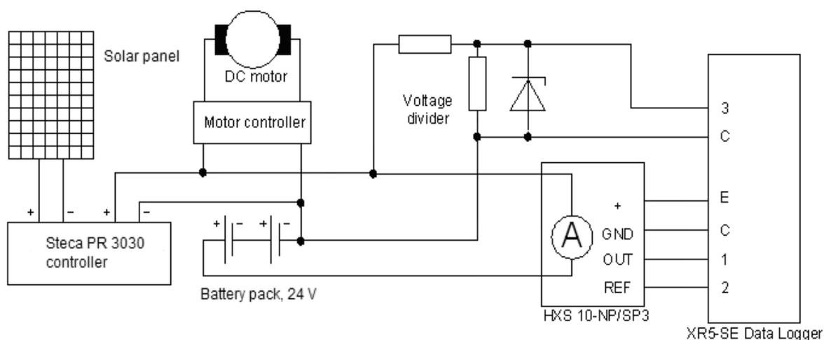
**Fig. 1. Principal Scheme of controller and measuring device connection**
