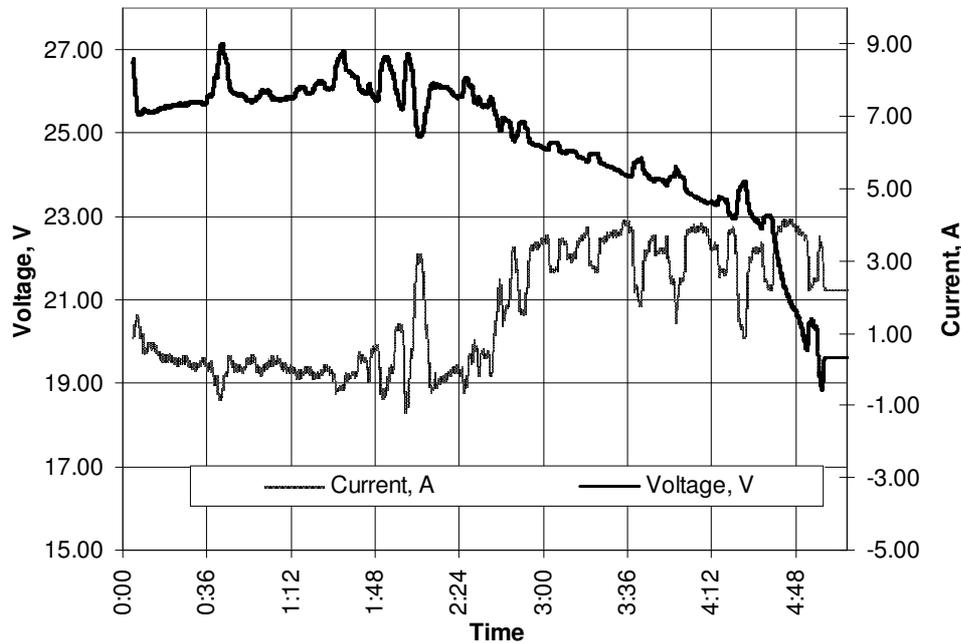
Fig. 2. Variations in voltage and current in the first experiment
