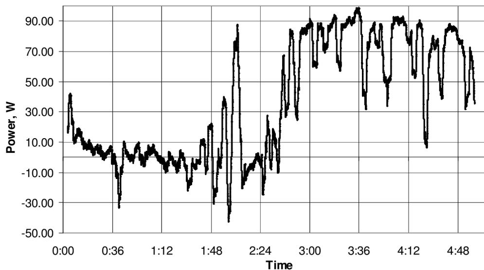
Fig. 3. Graph for the power released by the batteries in the first experiment
