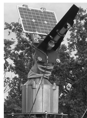
Fig. 2. Photovoltaic panel PVM10/12PF on the sun tracking stand EPR-203
