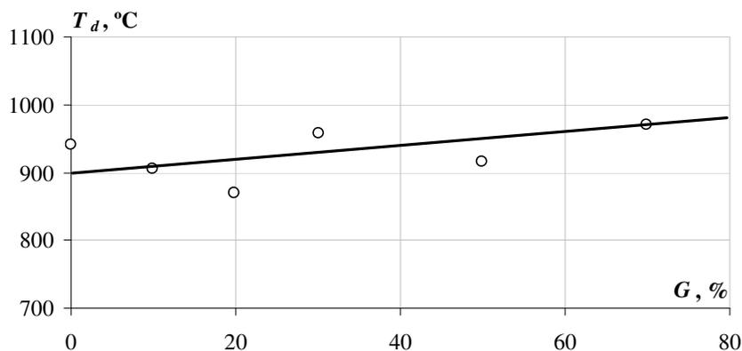
Fig. 2. Dependence of burning temperature  $T_d$  on the quantity of green glycerol in fuel blend  $G$  – comparative quantity of the blown air  $V_o = 5 \text{ m}^3 \cdot \text{kg}^{-1}$
