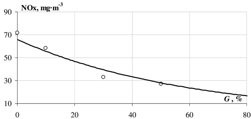
Fig. 3. Quantity of nitrogen oxide  $\text{NO}_x$  in smoke depending on green glycerol in fuel blend  $G$  – comparative quantity of air  $V_o = 5 \text{ m}^3 \cdot \text{kg}^{-1}$
