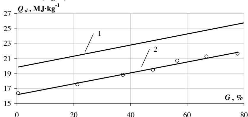
Fig. 1. Dependence of mixture of dry and wet sawdust and green glycerol calorificity  $Q_d$  on the quantity of glycerol  $G$  in it: 1 – calorificity of dry mass (calculated); 2 – calorificity of 8 % moisture blend (experimental value)
