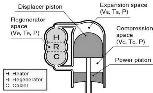
Fig. 1. Schematic illustration of beta type Stirling engine [13]
