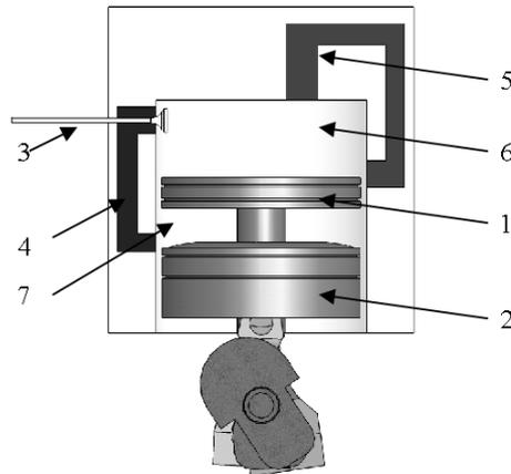
Fig. 2. **Schematic illustration of designed engine:** 1 – Displacer piston; 2 – Power piston; 3 – Valve; 4 – Cooler; 5 – Heater; 6 – Expansion space; 7 – Compression space
