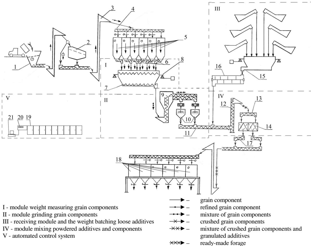
**Fig. 1. Flow diagram of a modular set of equipment:** 1 – receiving hopper; 2 – separator; 3 – elevator; 4, 13 – infeed conveyor; 5, 18 – bunker; 6, 17 – unloading conveyors; 7, 15 – weight bin; 8 – load cells; 9 – bin active; 10 – crusher; 11 – modular conveyor; 12 – vertical conveyor; 14, 16 – mixer; 19 – electrical cabinet; 20 – control cabinet; 21 – remote control
